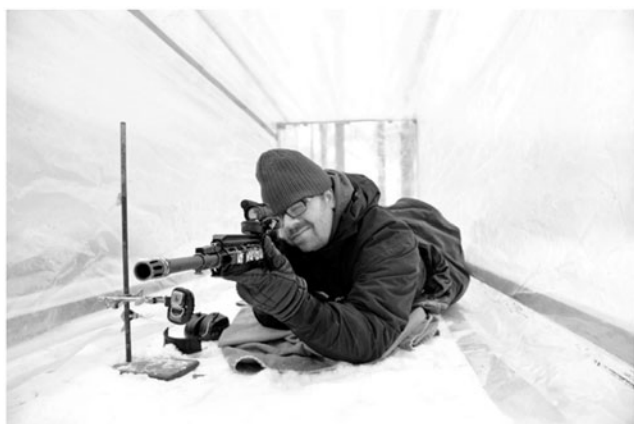
Figure 1. Shooter in a semi-airtight tent with HK416 and a CO sensor at the left (photo: NDRE).
