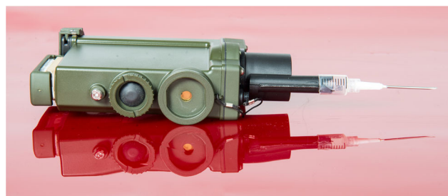
Fig. 1 LCD 3.1B detector connected to a survey nozzle and syringe with a 16G needle. This combination is here called the HS-LCD connection
