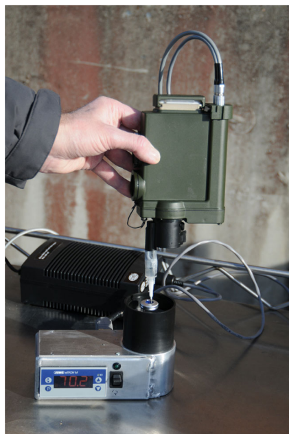
Fig. 6 A small and easy portable headspace vial heater used in the field experiments
