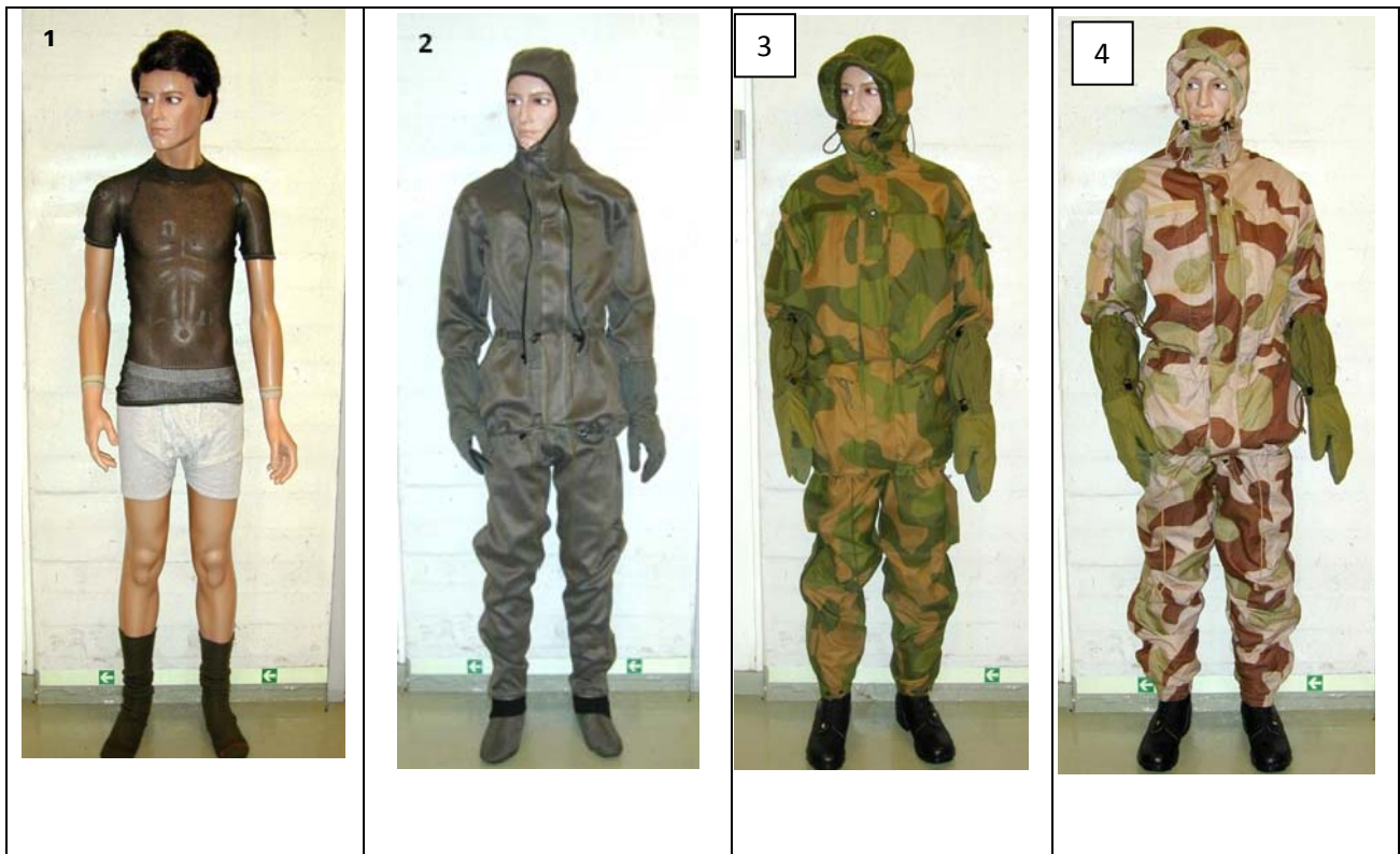
Fig. 1 The clothing layers worn in experiment 1. From left to right: 1: Underwear; 2: Charcoal layer (C-lining CD2880); 3: MEM and 4: TEX outer layer. Underwear (1) and charcoal liner (2) were worn under both the protective outer layers.
