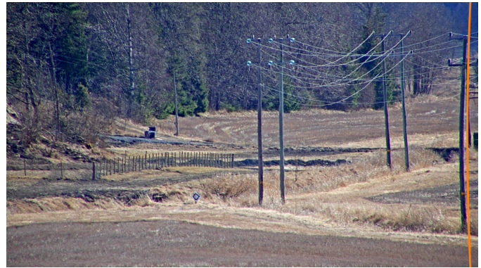
Fig. 14. A typical image from the real-world dataset. The 50\text{cm} \times 50\text{cm} april tag is approx. 550m away. The orange curve shows the distortion of a straight line with k = 70 at a horizontal FOV of 3.0^\circ . The power pole next to the curve is straight in reality, and appears to be even more distorted than the curve in this image.
