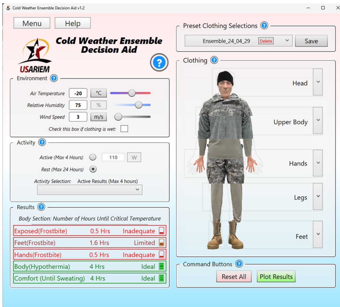
Figure 4. Example of a widely used decision support tool, cold weather decision aid (CoWEDA) that advises the number of hours that an individual can be exposed to a particular situation (environment, activity, clothing) before a potentially injurious temperature (body, hand, feet) is reached. Time to injury is based on skin temperatures reaching 5°C and core temperatures reaching 36°C.
