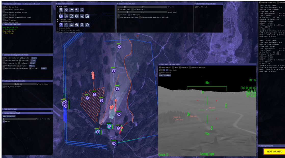
Figure 3.3 Valkyrie Ground Control Station (GCS), the interface for operating the swarm.
