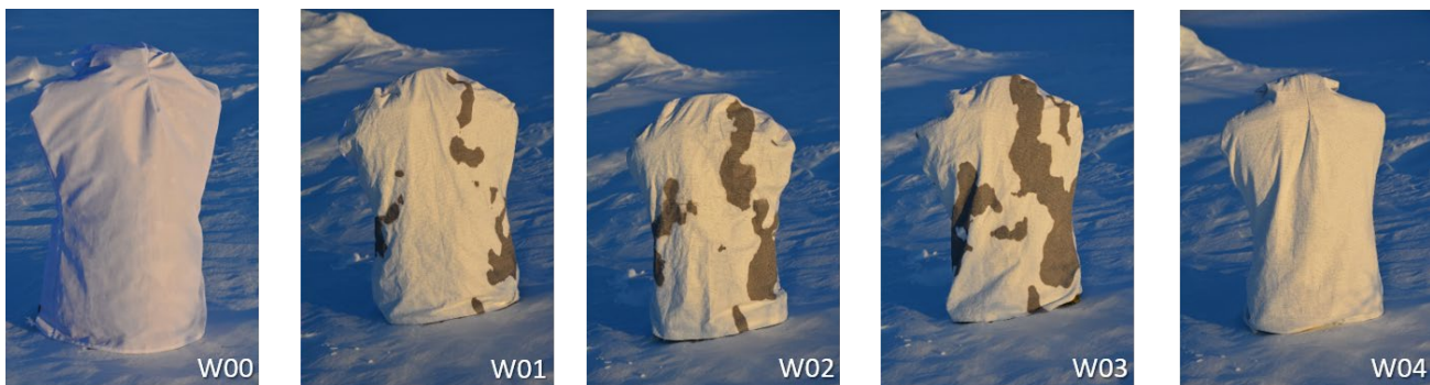
Figure 3. Winter camouflage patterns for evaluation in the visual range in Norwegian winter backgrounds. We captured the images at sunset, explaining the dark snow backgrounds dominated by shadows.
