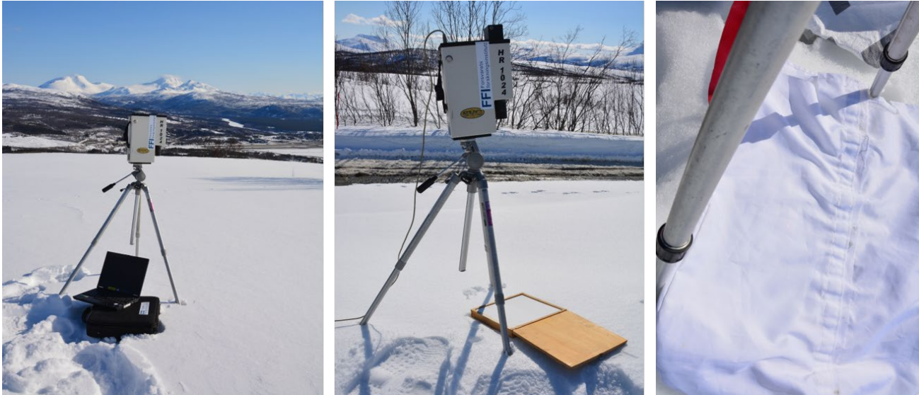
Figure 1. Measurement set-up for spectral measurements. Left: HR1024 spectrophotometer and a laptop for controlling the measurements. Middle: the spectrophotometer was calibrated using a white plate reflectance standard. Right: spectral measurements of a white textile.
