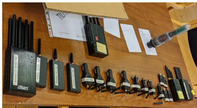
**Figure 2.** Twenty-one assorted jamming devices of various designs used throughout the PPD tests.
