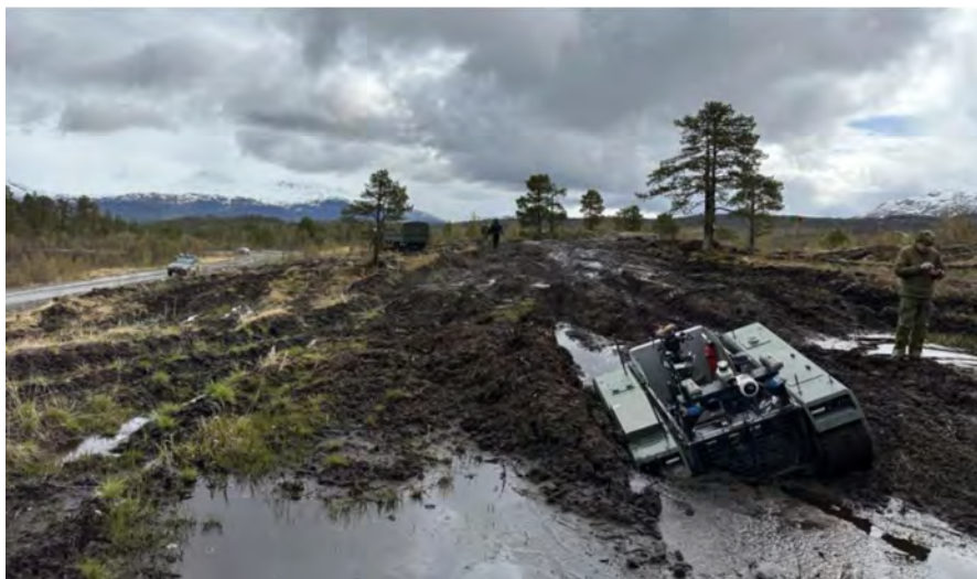
Figure 3.1 Top image: The UGV, Siv, firing with the Kongsberg remote weapon station. Bottom image: An UGV driven into a mud-pit because the operator misjudged the drivability of the terrain displayed on the video-stream.
