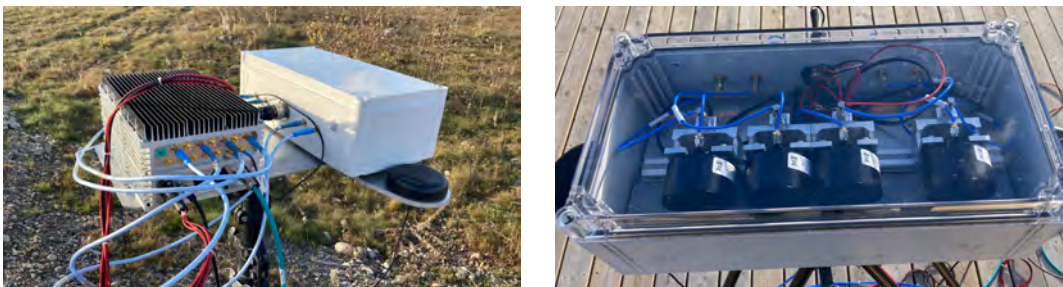
(a) An Elinor passive RF sensor node on LandX23 (b) The Elinor antennae with a bearing accuracy of approximately 0.1 degrees
