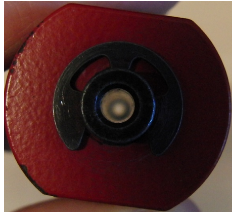
(b) The hole through the recoil booster.
