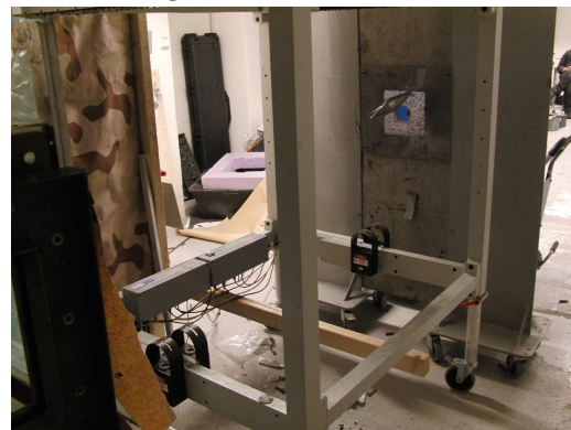
(c) Velocity detector and safety barrier.
