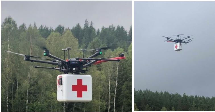
Figure 1.1 DJI Matrice 600 drone with a test payload for medical logistic services
