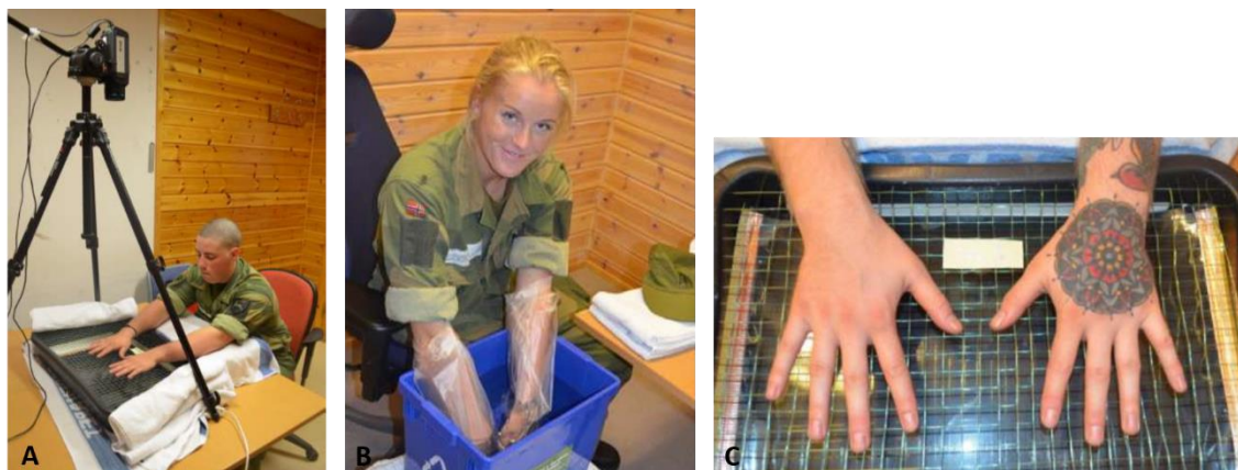
Figure 3.2 Photographs of the thermal experiment using Dynamic Infrared Thermography (DIRT) which was carried out during the conscript study in August 2014 and January 2015: A) right before cooling («Pre-cooling»), B) during the standardised cold provocation test with hands placed in a plastic bag reaching to the elbows and submerged in water up to the wrists for one minute in water temperature of 20°C ( \pm 1^\circ\text{C} ) and C) measurements every minute during the restitution phase (rewarming phase) for a total of four minutes with hands resting on a nylon grid. A heat source of 40 °C was placed 7 cm below the nylon netting. Photo: Arne Johan Norheim 2014/2015.
