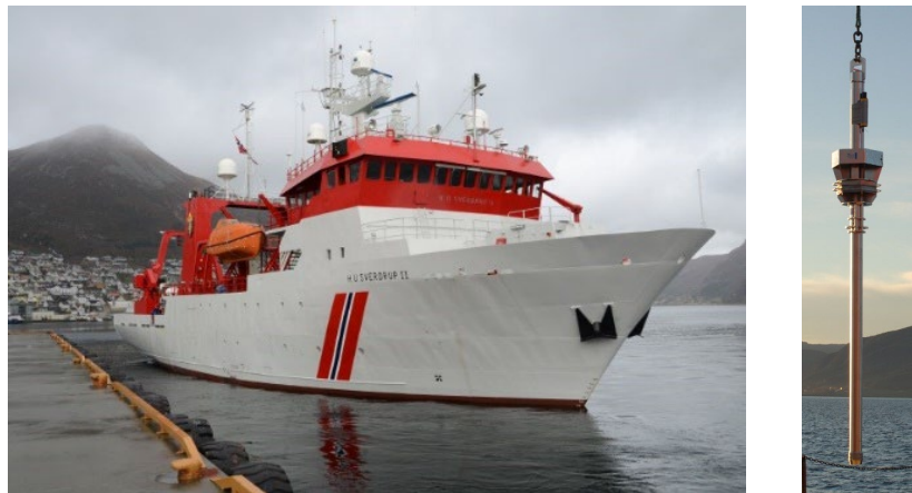
Figure 2. The cores were collected from the research vessel M/S H.U. Sverdrup II. The gravity corer from KC Denmark with a tube of length 2.5 m was used in the Norwegian Sea in 2013. Photos: FFI.
