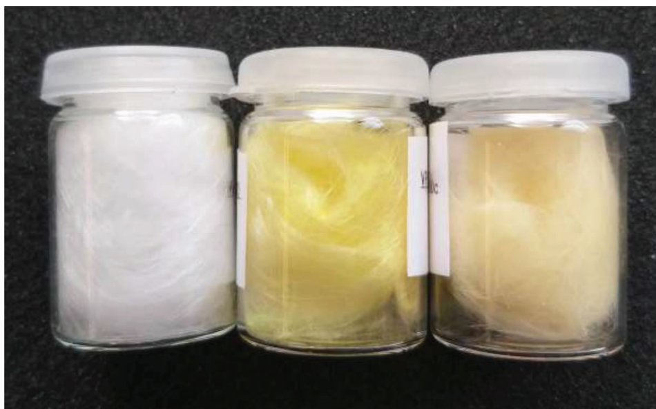
Figure 1. A photograph of the uncoated glass wool, as-deposited samples, and crystallized samples (from left to right). The yellow color is characteristic of UiO-66-NH 2 .
