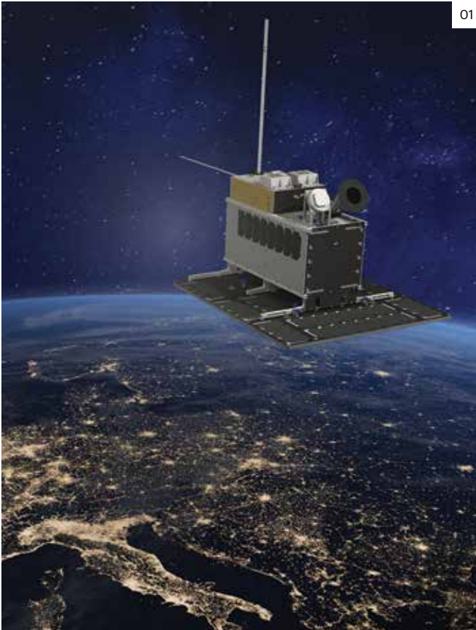
01 The FFI-developed radar detector for NorSat-3 will provide an even better overview of the shipping in Norwegian waters – including traffic that does not want to be detected. Photo: Norsk Romsenter / UTIAS / AdobeStock
