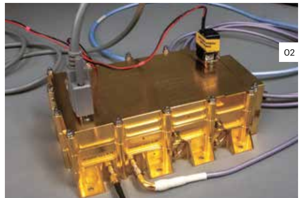
02 The ground penetrating radar RIMFAX is comprised of an antenna and a gold-plated box. The box contains the technology that enables it to ‘see’ what is hiding beneath the surface of Mars. Photo: Lars Aarønæs / FFI
