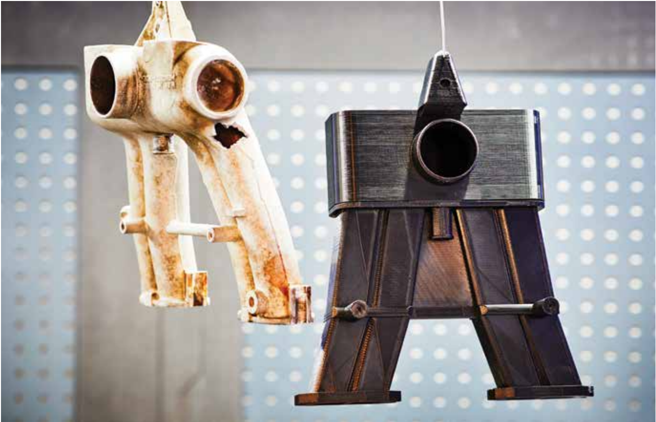
A worn part can be copied and produced on-site, when needed, within a very short period. Photo: Fieldmade
