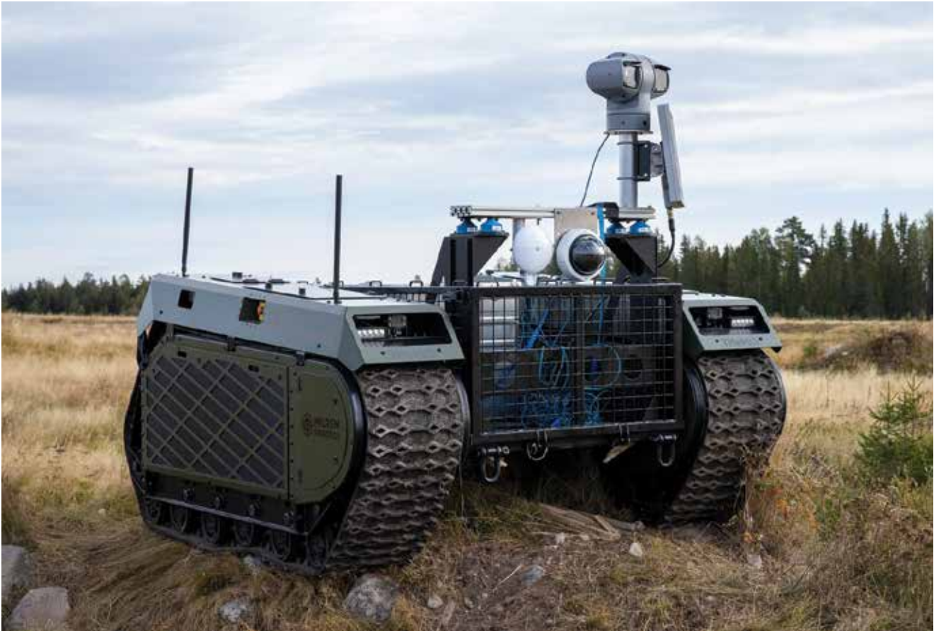
An unmanned vehicle with radar and pan-tilt-zoom camera is used to give the operator a better overview. Photo: Espen Wang-Naveen / FFI
