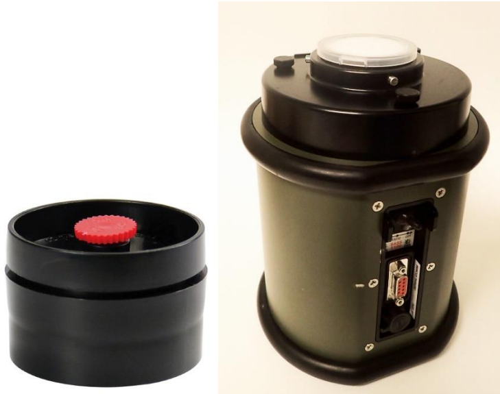
Figure 2.1 Conductive sampling cassette used for gelatine filters (left) and SASS 3100 air sampler with electret filter mounted on top (right).
