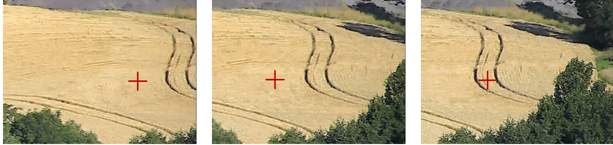
Figure 1: A fixed point in the platform frame projected into images from a PTZ camera where the image timestamps and pan/tilt timestamps are out-of-sync by about 50ms. The camera is panning to the right, and suddenly comes to a stop. The left and centre images are taken while the camera is panning towards the right. The right image is taken after the camera has stopped panning. On a properly synchronised and calibrated system, the projected point should appear fixed against the background.
