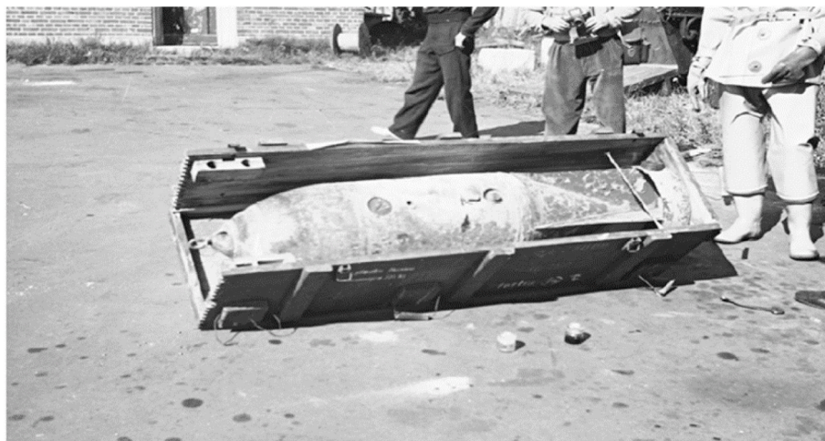
Fig. 1. Picture of a KC250 aerial mustard gas bomb (with permission from Bornholm museum).
