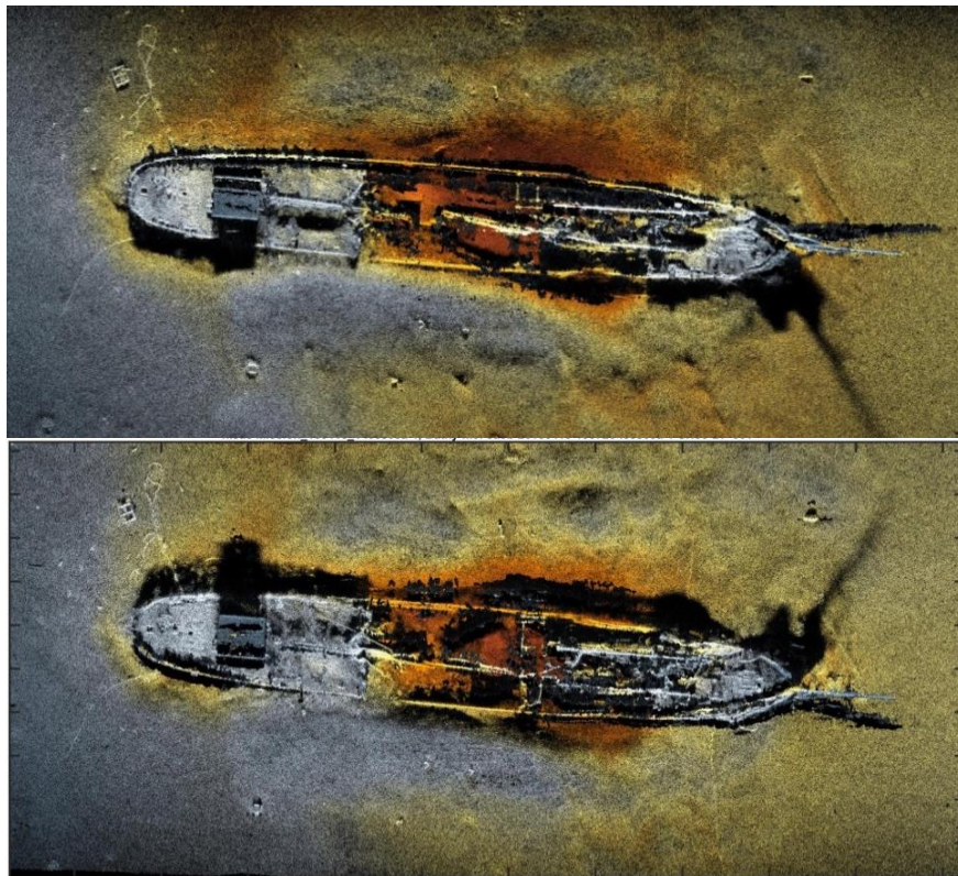
Figure 5.4 Fusion of SAS image and SAS bathymetry of a 90 m long sail ship in the Skagerrak strait. The wreck is not part of the CW dumpsite. Upper: Imaged from starboard side. Lower: Imaged from port side. The depth variation shown in the coloring is 5 m. Data courtesy of the Norwegian Coastal Administration.
