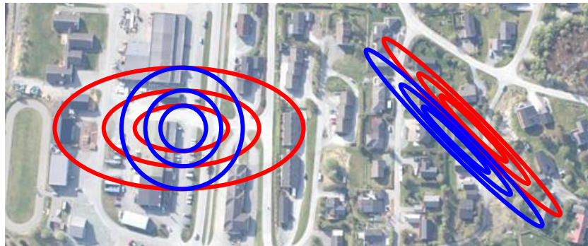
Figure 2. Illustration of the need for two-dimensional characterization of the PSF shape to determine coregistration. The contours illustrate PSFs of two bands in the same pixel, with a large coregistration error. Left: PSFs which appear to be equal when judged by a vertical LSF. Right: PSFs which have nearly equal LSFs in both horizontal and vertical directions. A characterization of coregistration from a single LSF may fail to detect the coregistration error in these cases.
