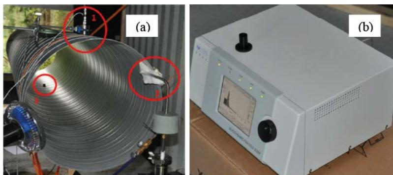
Fig. 4. (a)  $\text{\O}500$  mm duct through which the lidar was directed, and into which the aerosols were released either wet (1) or dry (2). (b) The APS measured the aerosol size distribution, and was located with its inlet protruding into the pipe (position 3 in Fig. 4(a)).
