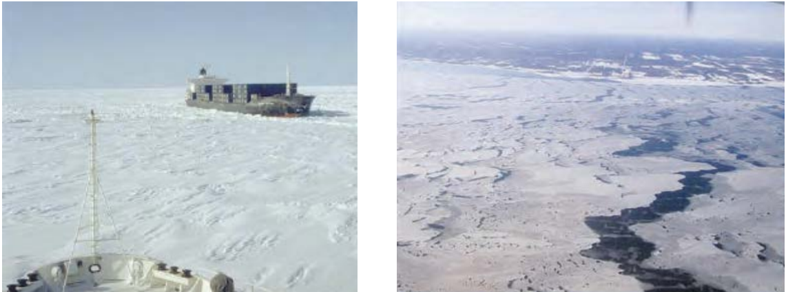
Figure 2.1 Left: Container ship tracking through a large pan of first-year ice. © Don Isaacs (CIS). Right: Very close pack light nilas and new ice. © C-GCFR (CIS)
