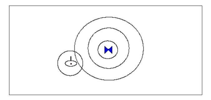
*Figure 3.2* Dynamics of submarine detection in OSCAR as illustrated by the concepts of sonar detection annuli and submarine noise circle.
