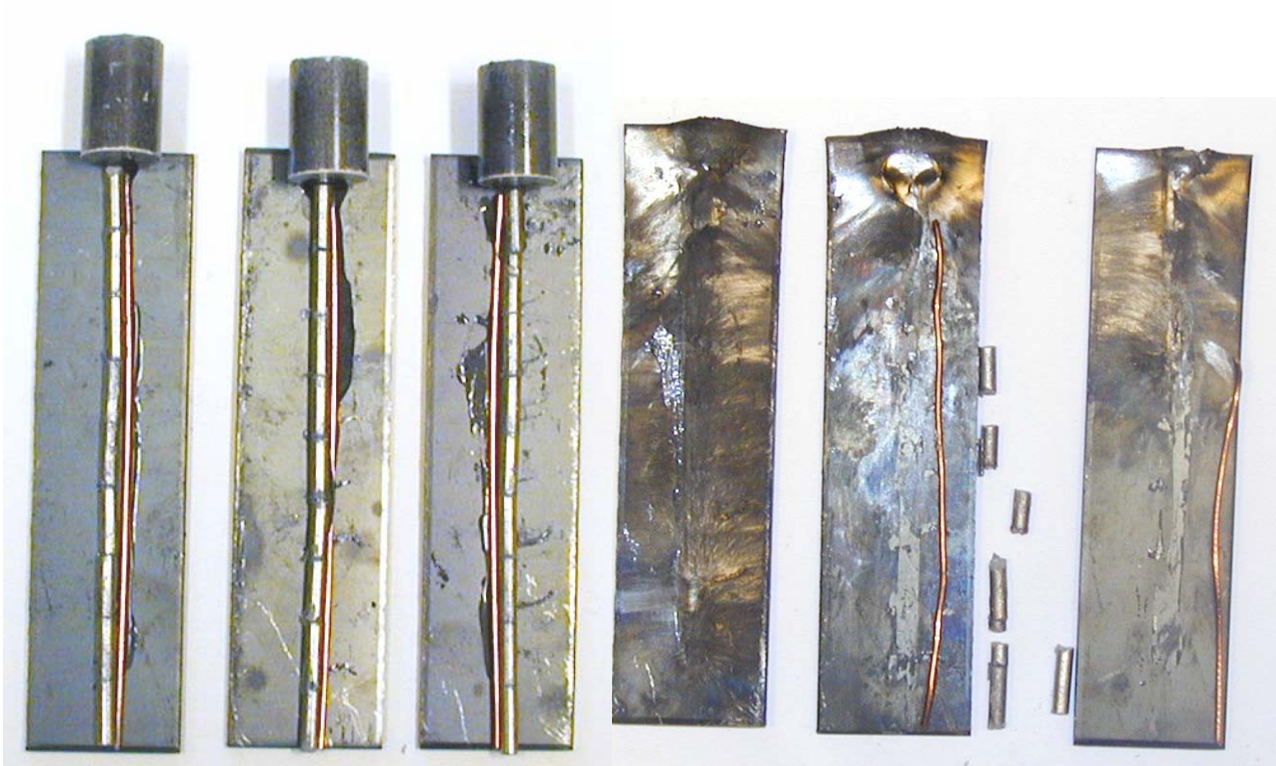
Figure 3.5 Pictures of charges used for testing of critical diameter, charge diameter 4.11 mm. The left picture shows the charges before testing and the right picture shows the witness plates after the charges were initiated.
