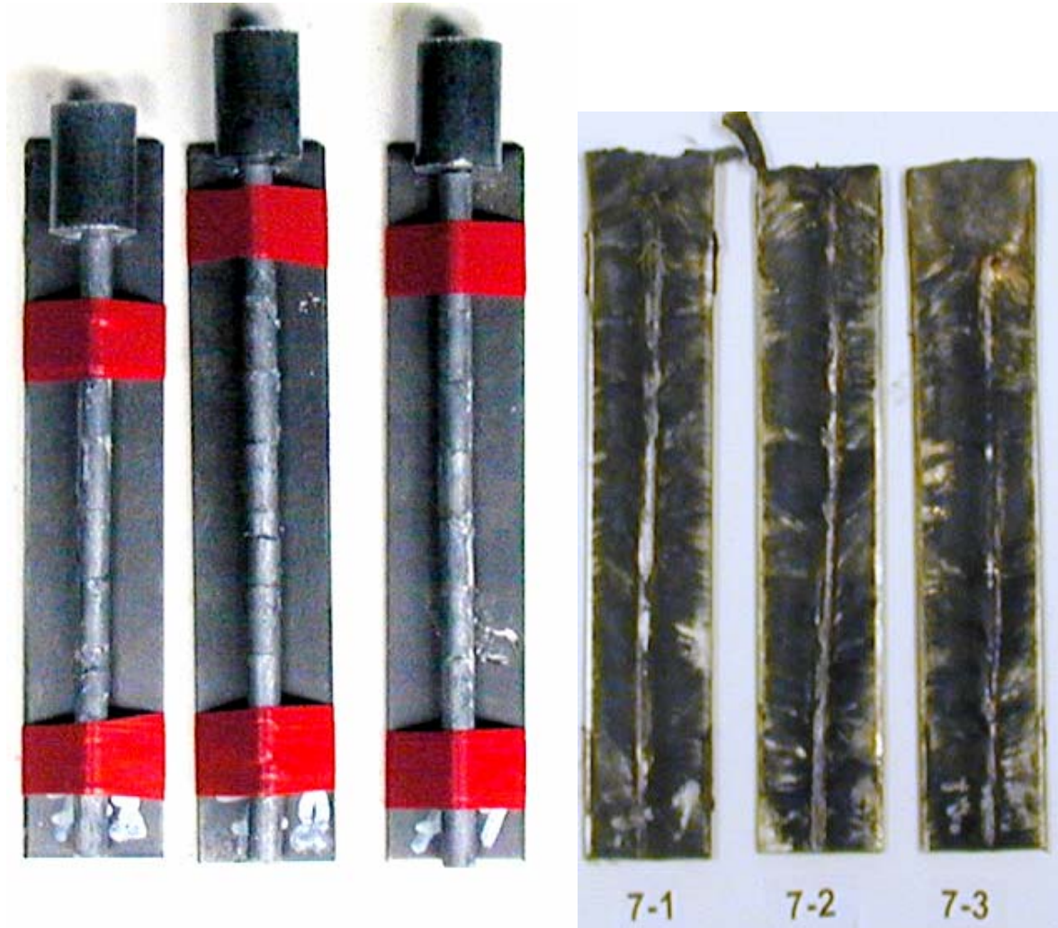
Figure 3.2 Pictures of charges used for testing of critical diameter, charge diameter 7.16 mm. The left picture shows the charges before testing and the right picture shows the witness plates after the charges were initiated.
