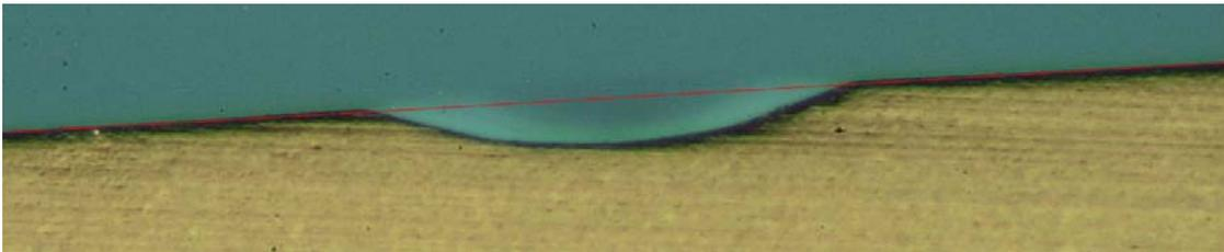
Figure 4.4: The indentation hole in Figure 3.4 seen from the side.
