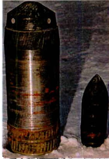
Figure 2.1: The 152 mm and 75 mm projectiles used in the HPC-experiments.
