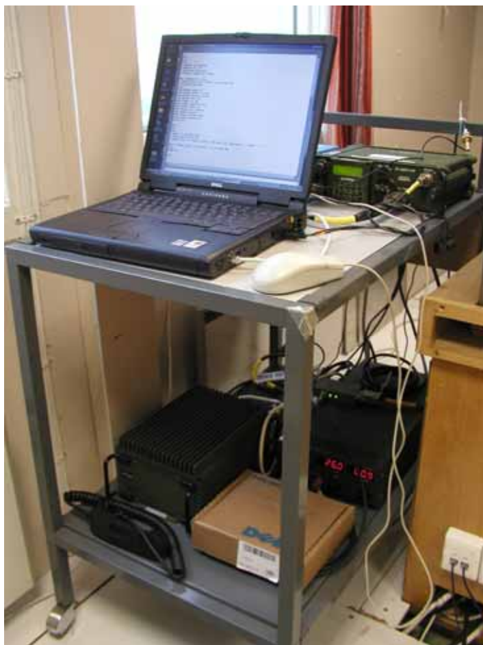
Figure 6 Test setup at each node in the network. RF-5800H, PC, 125 W Power Amplifier, power supply, PTT-box and Netgear router/modem
