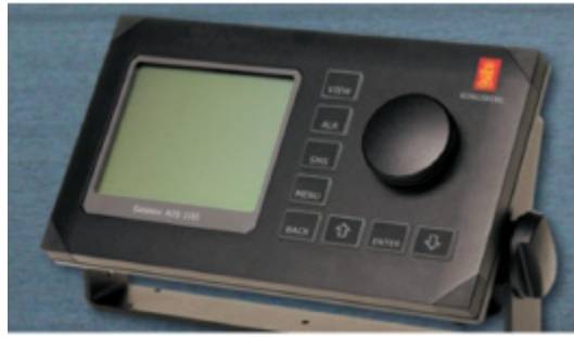
Figure 2.3 The Seatex AIS 100 mobile AIS station with an integrated display.
