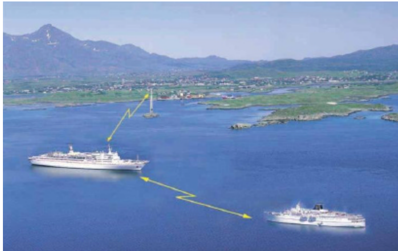
Figure 2.1 The AIS ship-to-ship and ship-to-shore concept. (Courtesy of Seatex, Norway).
