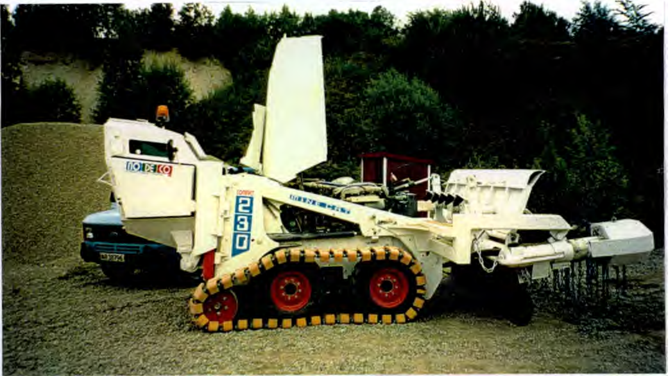
Figure 1.1 The Compact 230 MINECAT mineclearing vehicle, with hood open (Photo: NoDeCo)
