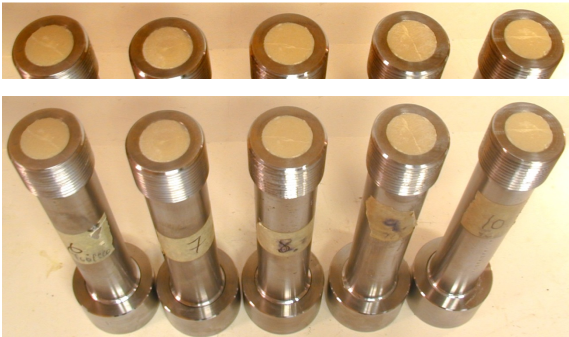
Figure 2.3 Pictures of tubes No 6 to No 10 after cleaning and modification of the end surface.
