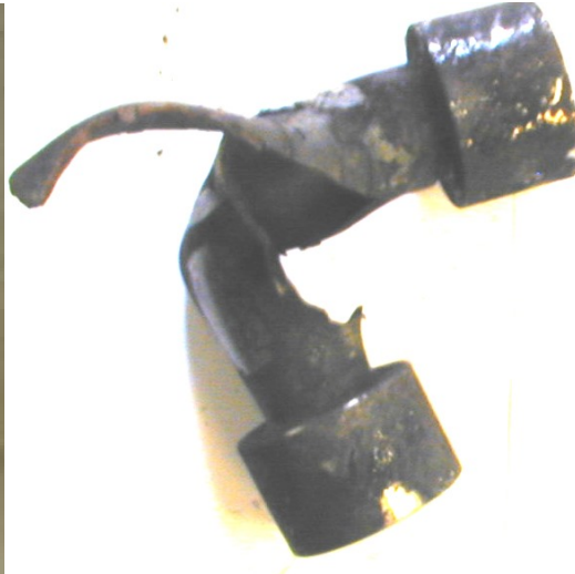
Figure 3.12 Picture of the recovered tube after testing.
