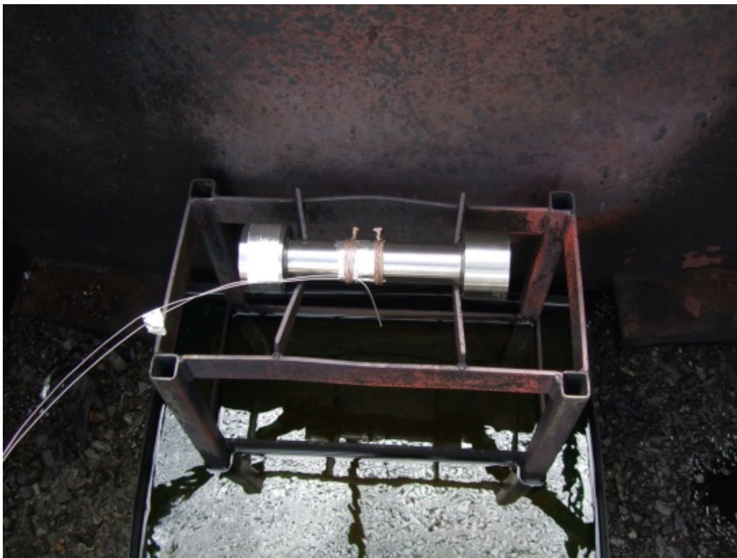
Figure 2.8 Test item with the two thermocouples seen from above.
