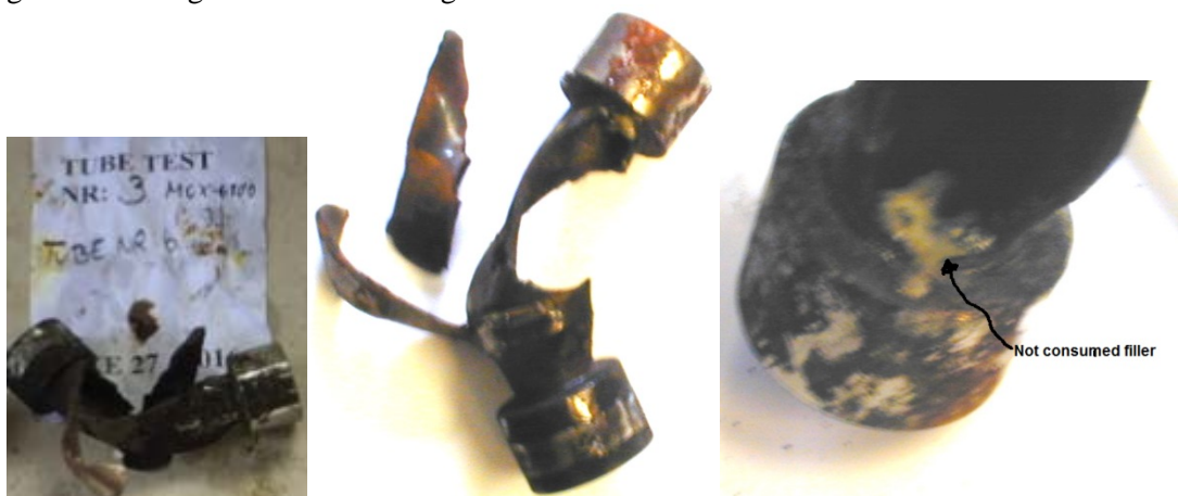
Figure 3.6 Pictures of the recovered tube after testing. Right picture shows recovered unreacted filler MCX-6100.
