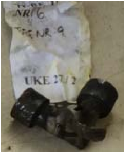
Figure 3.12 Picture of the recovered tube after testing.
