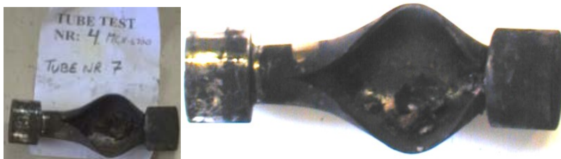
Figure 3.8 Pictures of the recovered tube after testing.
