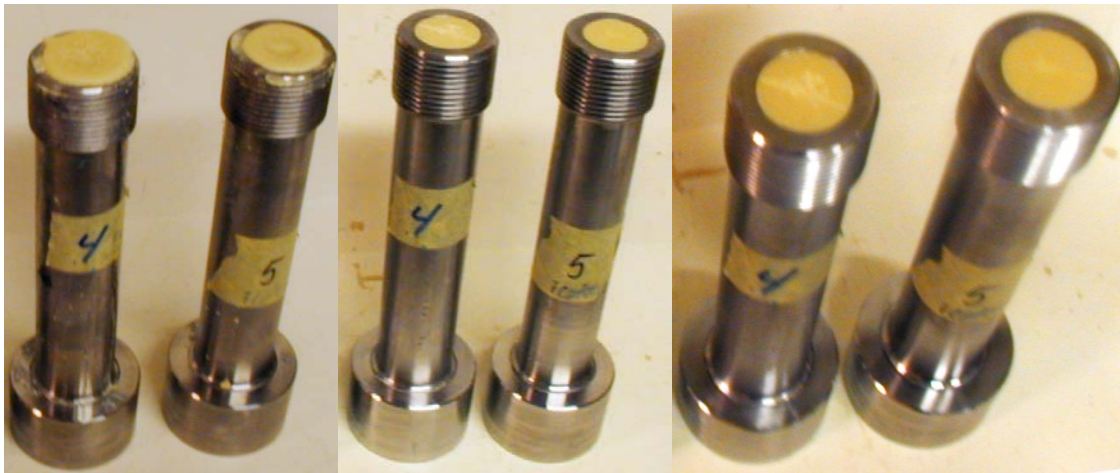
Figure 2.1 Pictures of tubes No 4 and No 5 as received from Chemring Nobel AS to the left and after cleaning and modification of the top surface in the center and to the right.
