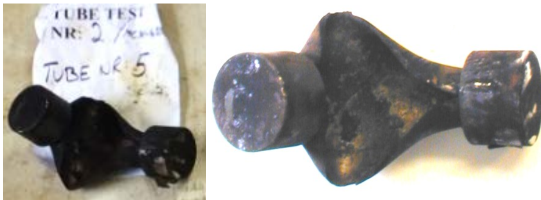
Figure 3.4 Pictures of the recovered tube after testing.
