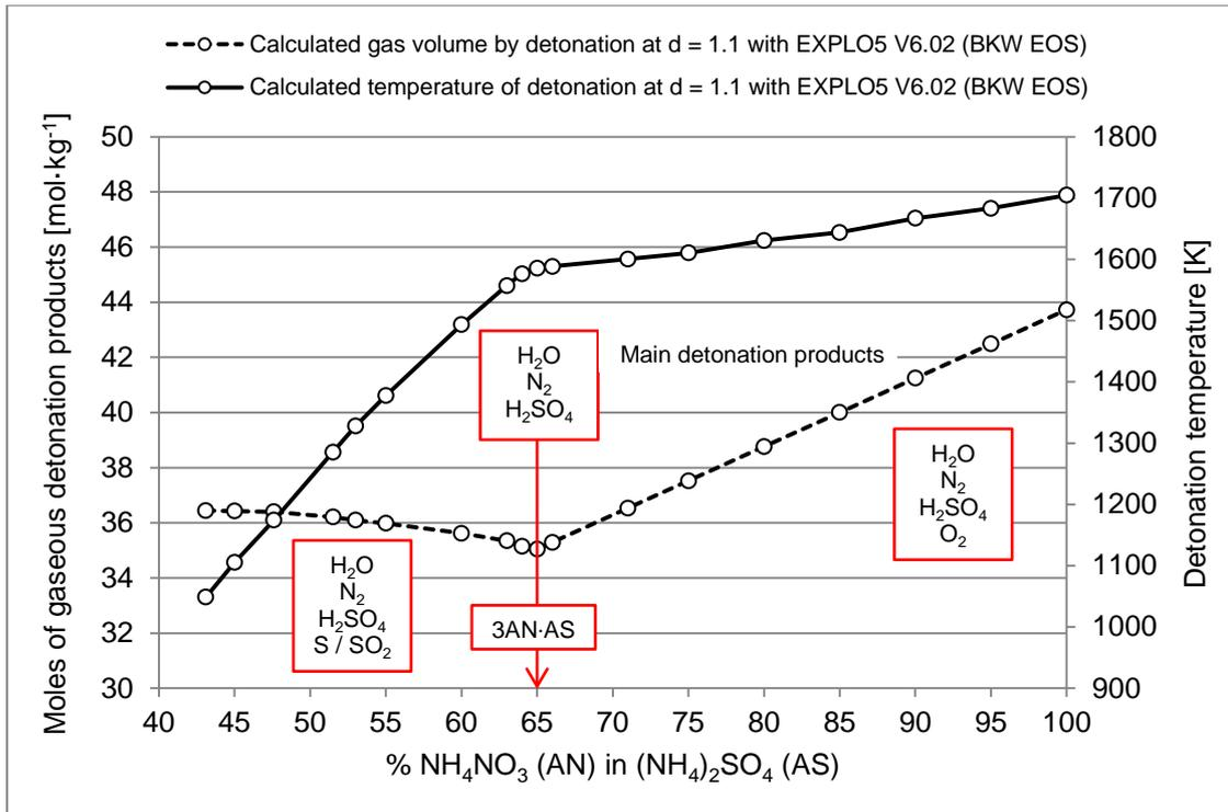
Figure 11.3 The quantity of gaseous reaction products and detonation temperatures of AN-AS mixtures calculated with EXPLO5 V6.02 at a constant density of  $1.1 \text{ g}\cdot\text{cm}^{-3}$  (using the BKW EOS). **Note:** Only the major reaction products are indicated.
