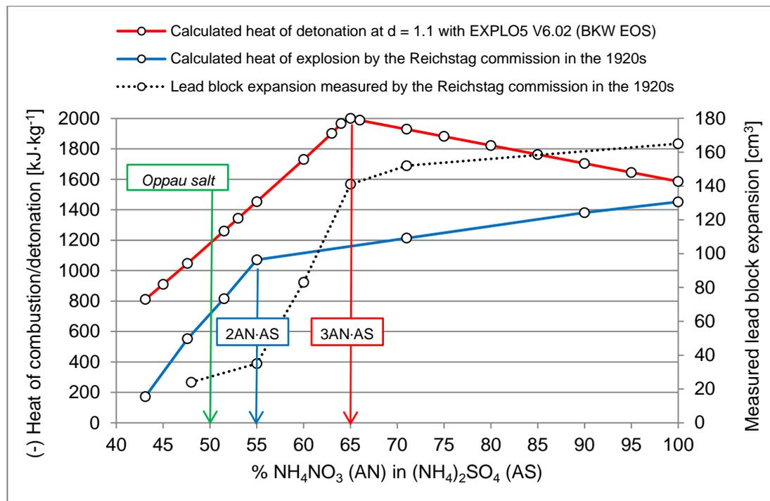
Figure 11.2 The (negative) heat of detonation of AN-AS mixtures calculated with EXPLO5 V6.02 at a constant density of  $1.1 \text{ g}\cdot\text{cm}^{-3}$  (using the BKW EOS) compared to the (negative) heat of explosion (combustion) as calculated by the Reichstag commission in the 1920s. The experimental lead block expansion values (with the contribution from the detonator included), measured by the Reichstag commission for such mixtures, are also plotted.
