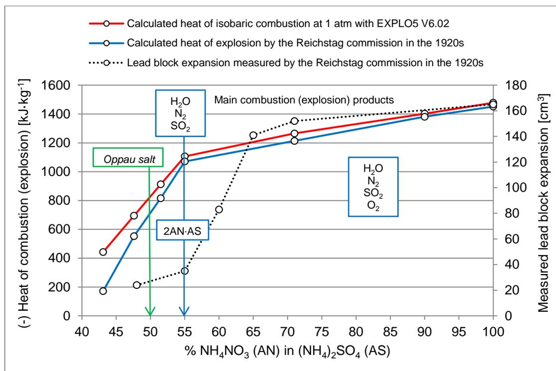
Figure 11.1 The (negative) heat of explosion of AN-AS mixtures as calculated by the Reichstag commission in the 1920s (blue line), compared to the (negative) isobaric heat of combustion of the same mixtures calculated with EXPLO5 V6.02 (red line). The experimental lead block expansion values (with the contribution from the detonator included) measured by the Reichstag commission for such mixtures are also plotted (dotted line). **Note:** Only the major reaction products are indicated.
