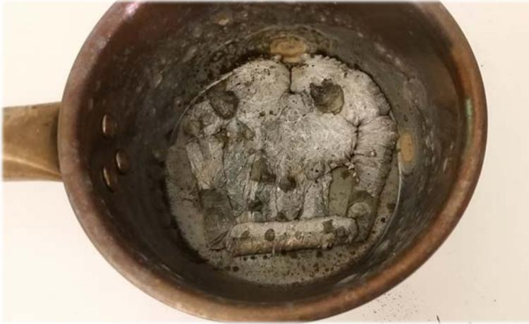
*Figure 2.5 Resulting pot after the first direct addition experiment revealing deformed aluminum pieces.*
