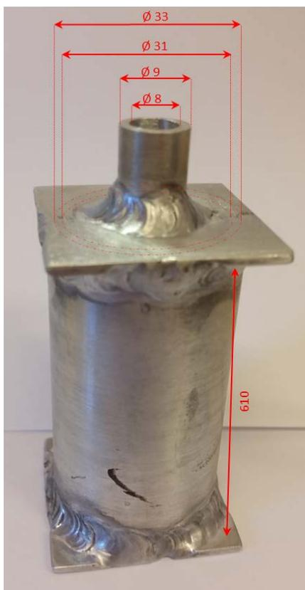
*Figure 2.6 Down-scaled vented pipe test-tube with appropriate measurements in mm.*
