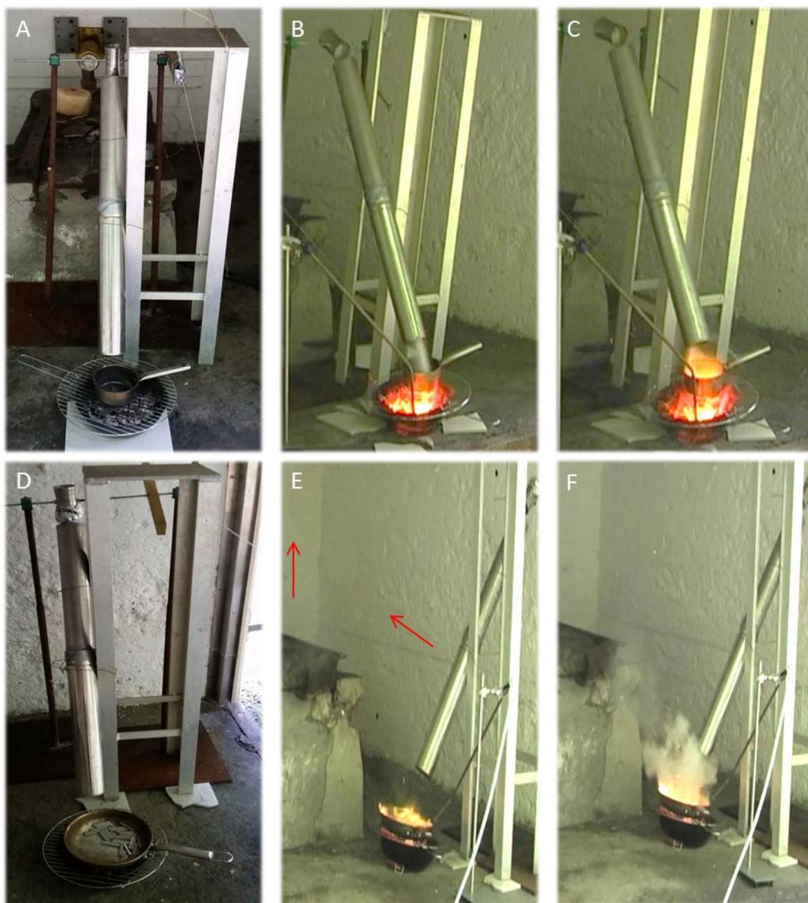
*Figure 2.4 A) Experimental set-up with steel pot; B) Addition of ANPP to melted aluminum; C) Shooting flames appear after 10 seconds; D) Experimental set-up with steel pan; E) Flames light up immediately after addition of ANPP. Orange-brown fumes can be seen, as indicated by the red arrows; F) The vigorous flames are replaced by the decomposition of AN yielding water fumes.*
