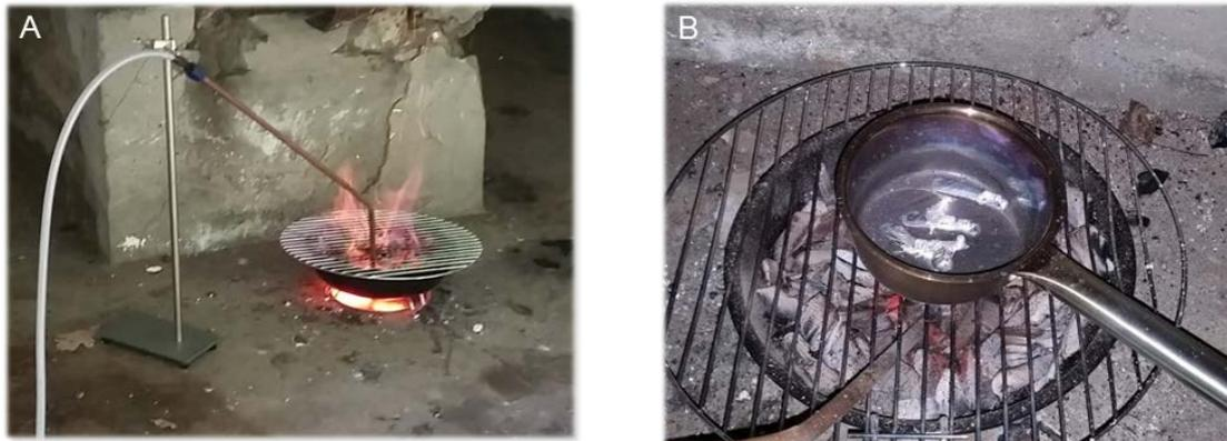
Figure 2.1 A) Furnace set-up using a commercial barbeque, wood charcoal and an air compressor; B) Aluminum melt.
