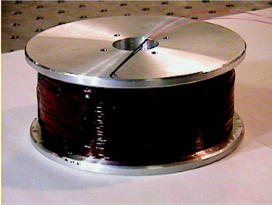
Figure 3.5: Aluminium spool with epoxy (stycast) glue
